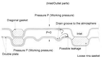
The *Ameri-Safe* cassette system provides an extra margin of safety due to the design of the cassettes with leak channels to the atmosphere. This ensures instant and readily apparent leakage detection capability.
